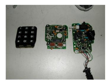
Here are the three circuit boards removed from the case. Left to right are the keypad, the DTMF generator board, and the microphone audio board.
