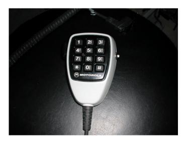
This photo shows the finished microphone. I took a small pair of diagonal cutters and trimmed the handle on the switch so that only enough protrudes to make it easy to activate.
