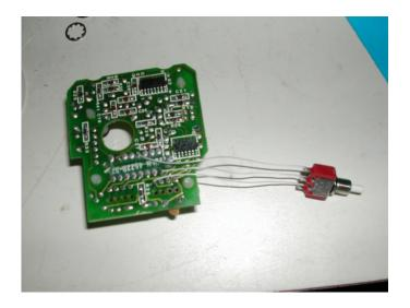
Here is the switch wired to the board. Note: The common pin is NOT connected properly in this photo...verify with ohmmeter that you have the correct pin on the keyboard connector. I took the photo before I found the mistake!
