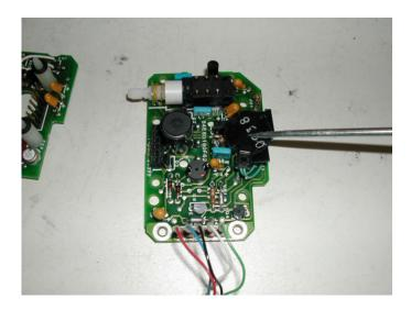
To improve the microphone audio quality, change R19 to 100K and change C2 to .047uF. R19 us near the bottom edge of the board just above the white wire. C2 is just to the left of the "beeper".
