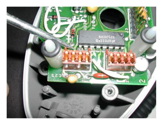
Cut the trace on the board indicated by the pointer. This breaks the connection from column 3 of the keypad to pin 5 of U2.
